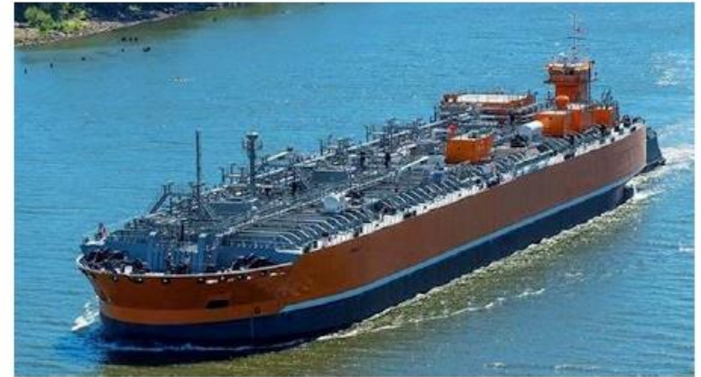
Refrigerated ammonia barge (image: Vigor)
